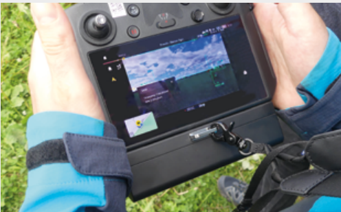
Drone remote control equipped with a bright 7-inch screen
